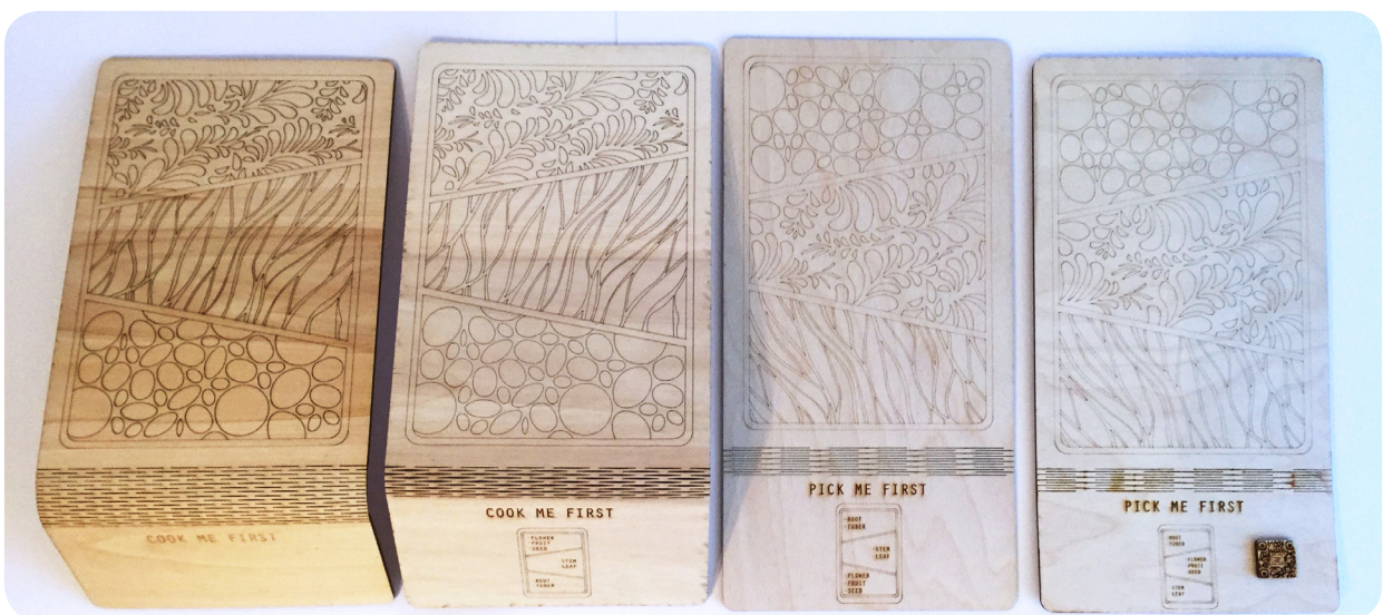
Figure 46. Tests of the living hinges, size and pattern modification of the lid. The right output was chosen as the final prototype.
