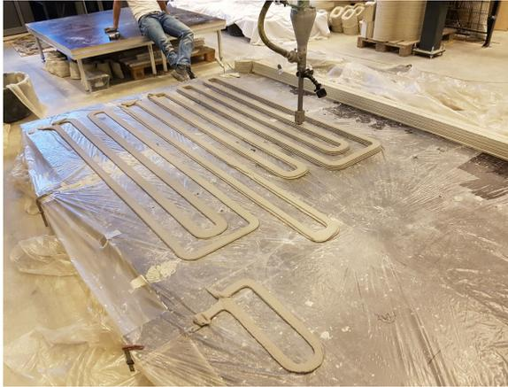
Figure 4.1: Printing table with final printed elements with one, two, three and four layers.
