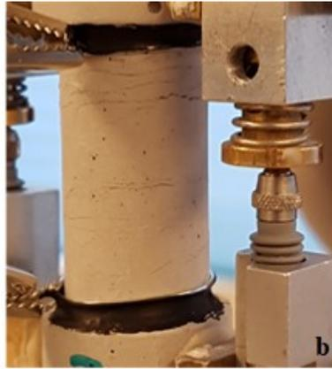
Figure 7.4: Multiple cracks developed during tensile test.
