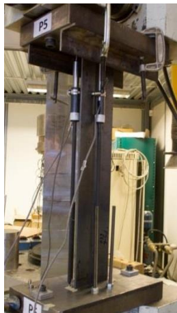
Fig. 3 Set-up for the compression tests
