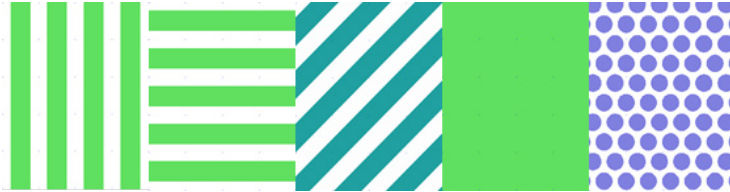
FIG 5. 14 Patterns in the calibration sample; the color part is electron transparent area, and the white is tungsten. Lines: 0.5\ \mu\text{m} wide, 1\ \mu\text{m} pitch; holes: 0.4\ \mu\text{m} diameter, 0.6\ \mu\text{m} pitch.
