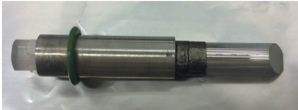
FIG 5. 10 The Optical fiber imaging conduit in an aluminum tube to seal vacuum; its 45o cut end is coated with a 50 nm aluminum layer.
