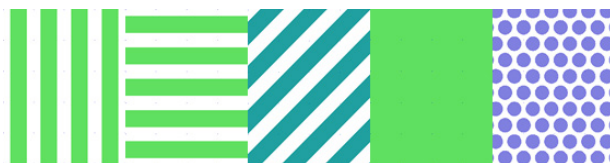
FIG 3. 6 Calibration sample; the color part is electron transparent area and the white is tungsten. Lines: 0.5 \mu\text{m} wide, 1 \mu\text{m} pitch; Holes: 0.4 \mu\text{m} diameter, 0.6 \mu\text{m} pitch.
