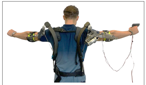
Figure 9: The manufactured semi-passive prototype worn on the right arm versus the conventional passive exoskeleton worn on the left arm.
