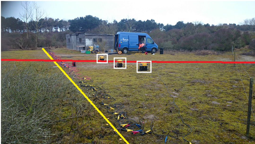
Figure 3-3: Picture of the field set up, yellow line and red line denote respectively line 1 and line2. The geodes are denoted by the white rectangles.
