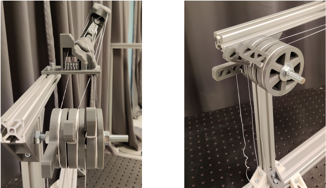
Figure 5.3: Lever-based actuation system for joint motion control.
