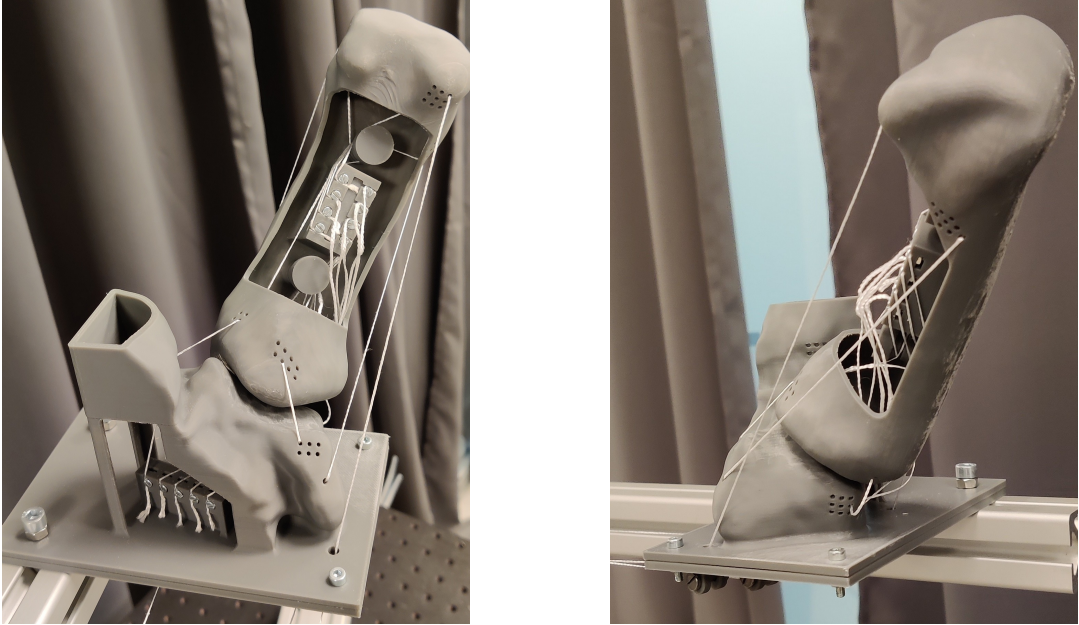
Figure 5.2: Frame assembly with the 3D-printed trapezium and metacarpal model mounted in place.
