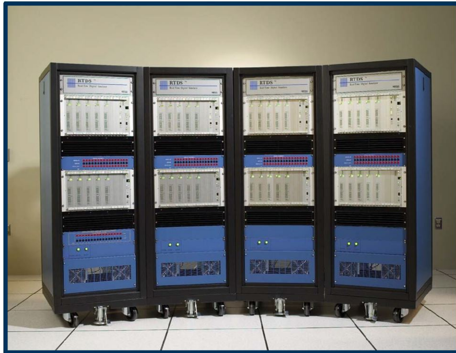
Figure 3.1: The RTDS Power System Simulator ( www.rtds.com ).
