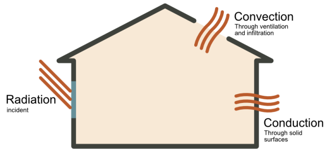
Figure 15 Different ways of heat transfer through building envelope modified from (Archi-Monarch, n.d.)
