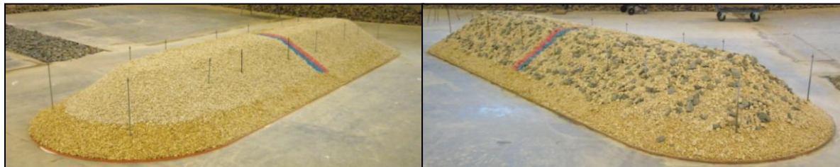
Figure 5: Final results of the mixtures on the breakwater model
