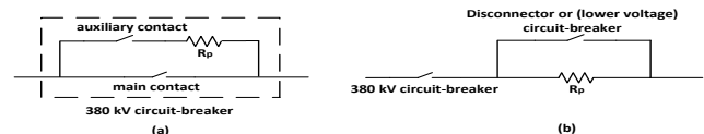
Fig. 16. Use of resistors to mitigate the zero-missing phenomenon, (a) a circuit-breaker equipped with the pre-insertion resistor, (b) a resistor in series with an ordinary circuit-breaker.
