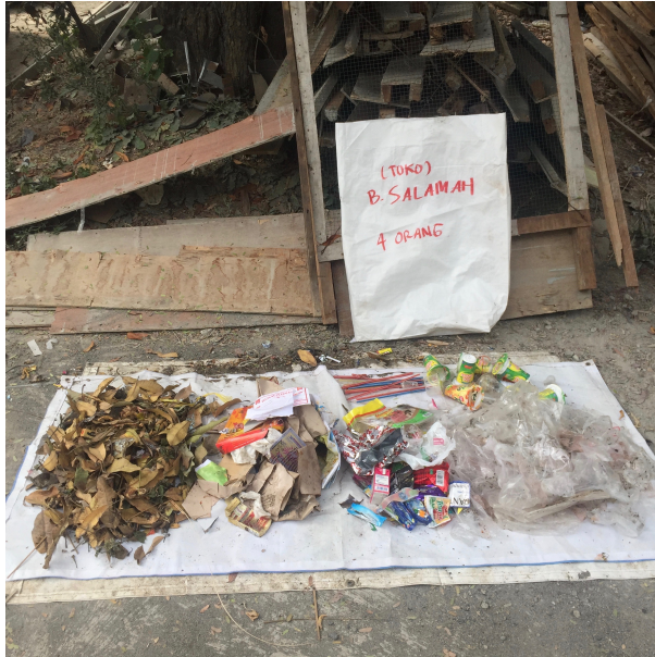
Figure 51: Household waste from one day is sorted and there-after weight per category
