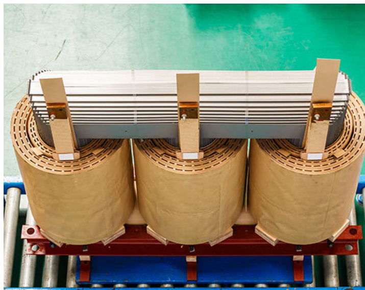
Figure 2.7: This figure shows the inside components of a transformer. The grey part is the transformer's core, through which the magnetic flux passes. The brown parts are the windings encircled with paper for better insulation. There are holes in the paper to have oil circulating more closely around the windings [19].
