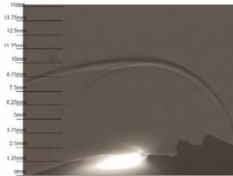
Fig. 2.5: Phase-averaged schlieren image of compression waves generated by NS-DBD plasma actuator viewed along the major axis of the discharge a 30 cm DBD load.[58]
