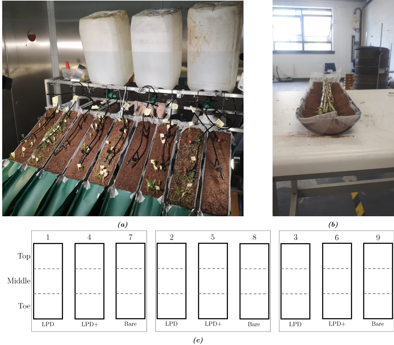
Figure 2.3: Front view of the lab experiment setup. (a) Photo of the setup. (b) Position of the LPD bundle in a gutter before it is covered with soil. (c) Schematic drawing of the setup. LPD: gutter with soil and a LPD bundle; LPD+: gutter with soil, a LPD bundle and alfalfa seeds; Bare: gutter with only soil.
