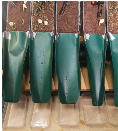
Figure B.5: Installation of the funnels which redirect runoff.
