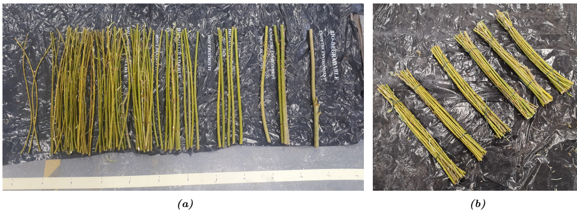
Figure B.2: Preparation of the bundles. (a) Sorting of the willow cuttings according to diameter. (b) The assembled bundles, tied tightly.
