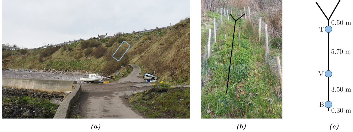
Figure 2.1: Layout and location of the LPD. (a) The slope in which the LPD was installed. The LPD is located within the box. (b) View from the bottom of the slope with LPD. The black lines indicate the centre of the LPD. (c) Locations of testing and sampling along the LPD. T: top, M: middle, B: bottom. The values are the distances between the locations measured along the slope.
