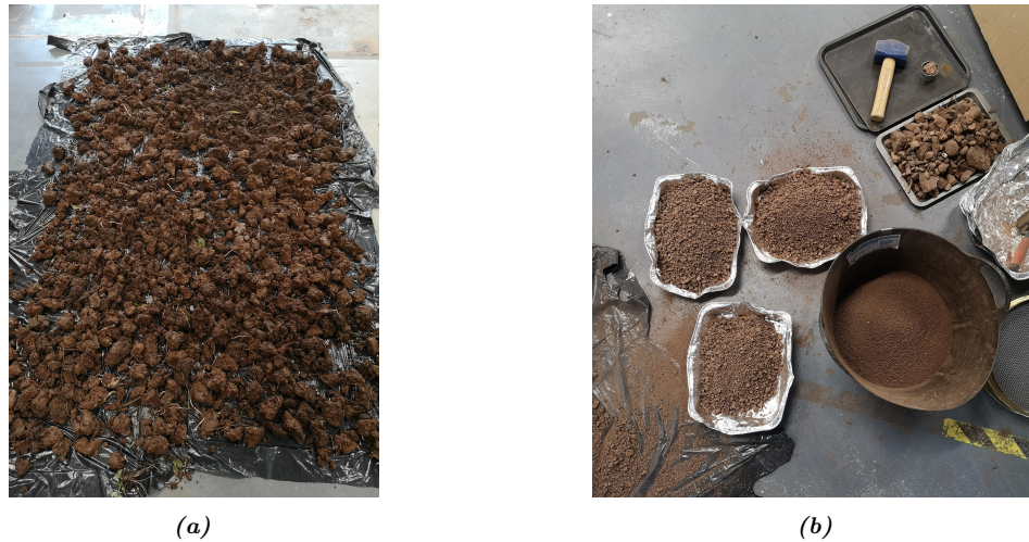
Figure B.1: Preparation of the soil. (a) Air drying. (b) Hammering and sieving of the soil.
