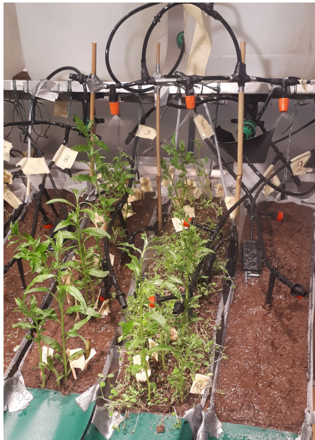
Figure B.8: Precipitation simulation setup.
