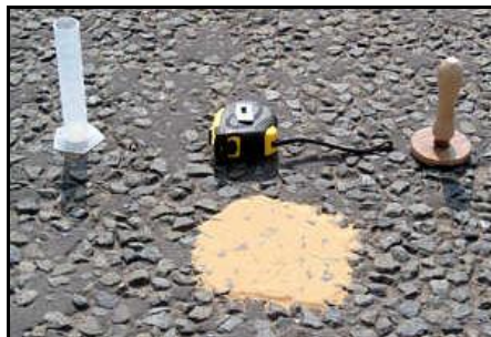
Figure 3-6: Sand patch measurement method (Source: highwaysmaintenance.com).
