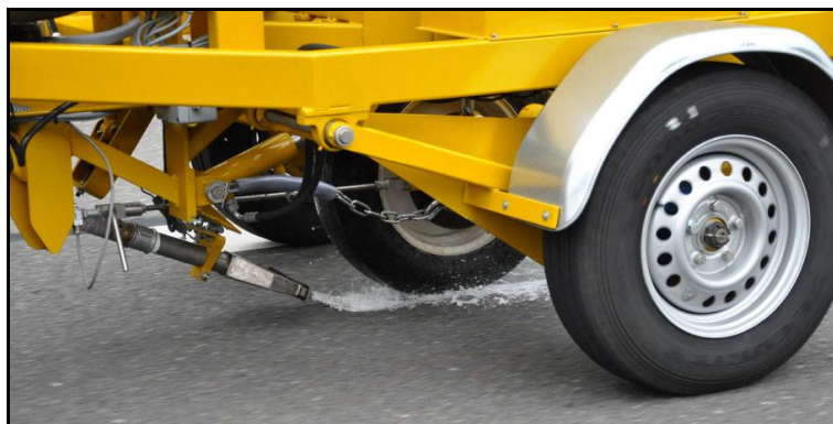
Figure 3-2: Skid resistance measurement method (KOAC-NPC).
