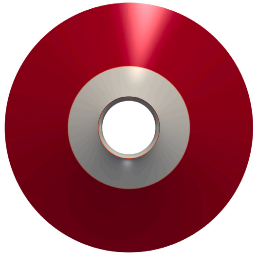
(d) Top view of the deformed annulus using the tension field theory membrane model. The red region denotes a taut, and the gray region denotes a wrinkled region.
