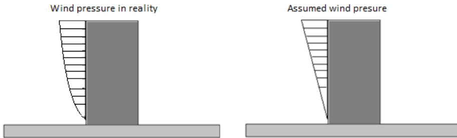
Figure 46: Wind load in reality versus assumption of the wind load acting on a building
