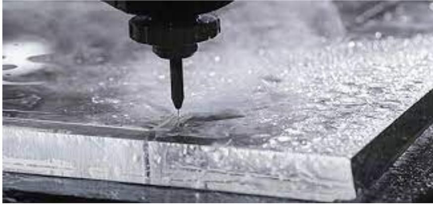
Figure 30: Water jet cutter
