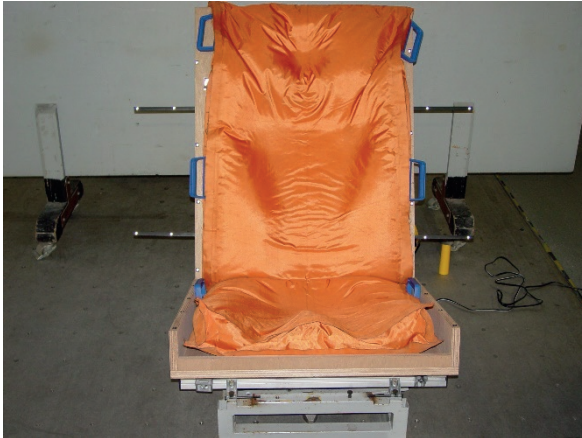
Figure 24: Frame with vacuum mattress after imprinting in the lab.
