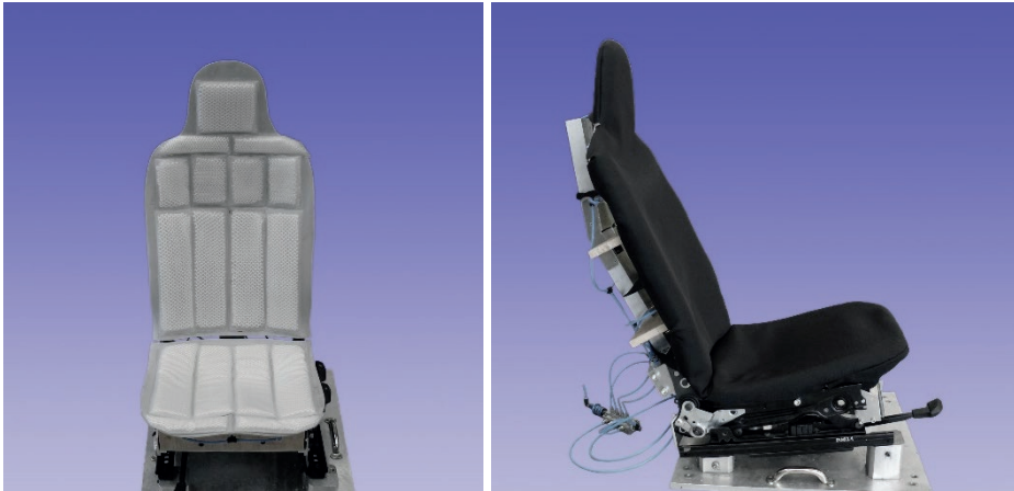
Figure 28: Prototype of the light weight body contoured seat. Left: the inflatable cushions.
