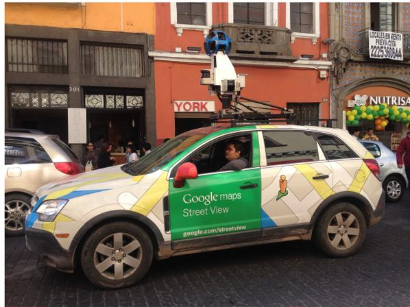
Figure 6.5: Example of multiple camera setup being used by google to gather streetview panorama images. Multiple cameras are located in the blue ball on top of the car. The sick modules are for lidar, a technique used for depth mapping. Courtesy of [41]
