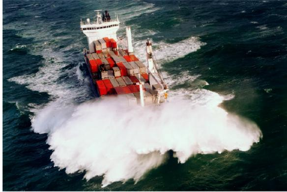
*Figure 1.2: A ship in waves, experiencing wave impacts.*
