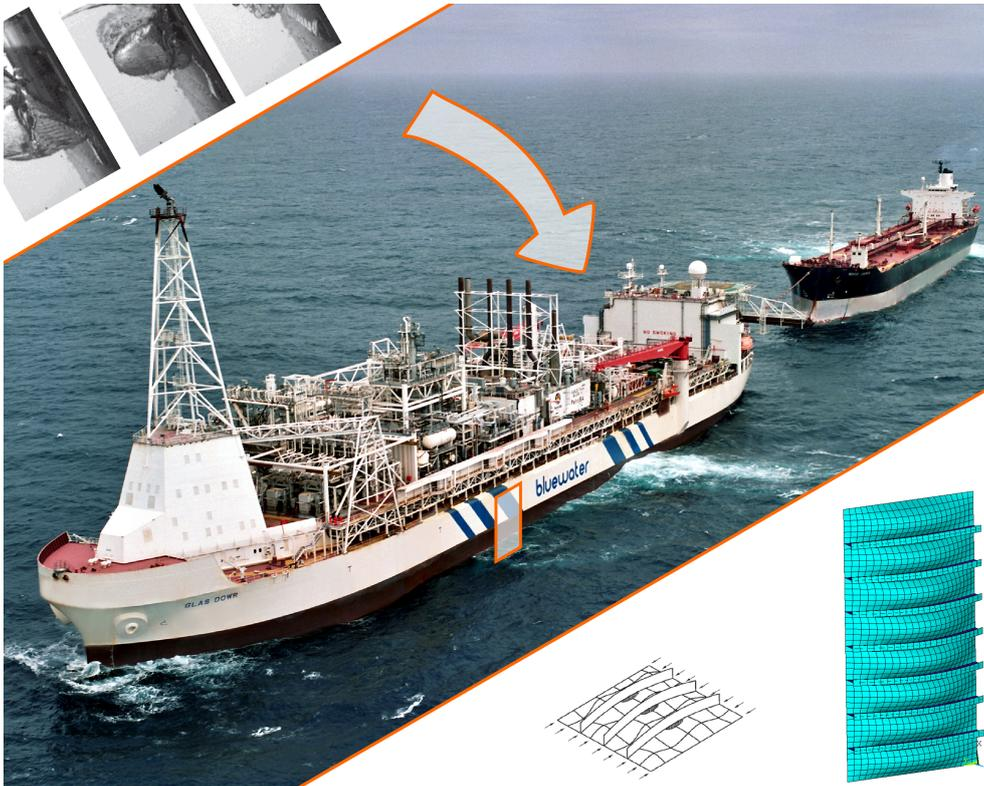
**Figure 1.1:** An FPSO in offloading condition<sup>1</sup>. Top left corner shows three wave impact loads from Guilcher et al. 2014, bottom right corner a limit state of Paik and Thayamballi 2003b and a stiffened plate field: the structure under consideration in this work.
