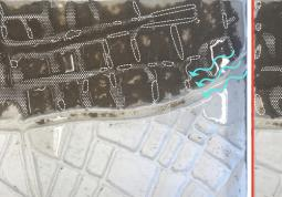
OCurrent state with demolished The main erosion happens around the linear dykes while the conjunction part remains.
