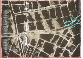
River comes into the flood plain 2 More sediments in the ponds 3 The final sedimentation pattern around dyke
