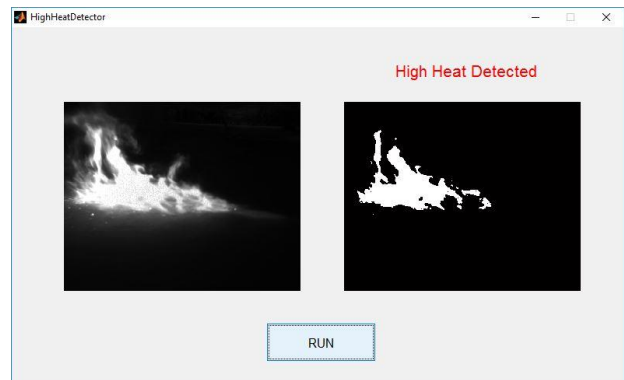
Figure 9: Detection of high heat using thermal imaging
