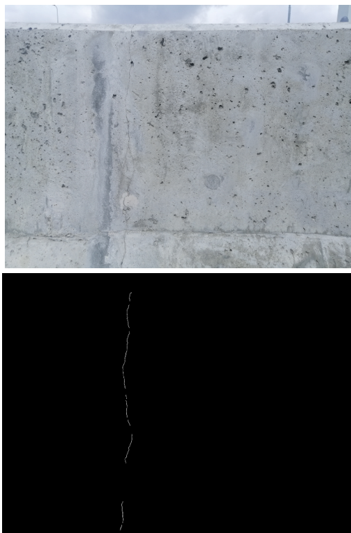
Figure 3: Example of image and corresponding segmentation mask (white pixels - crack, black pixels – background)
