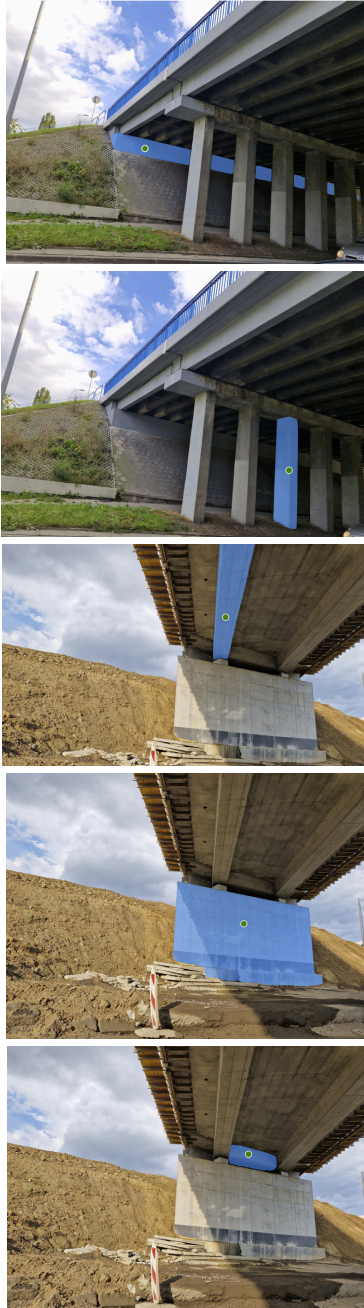
Figure 7: Results of bridge element segmentation
