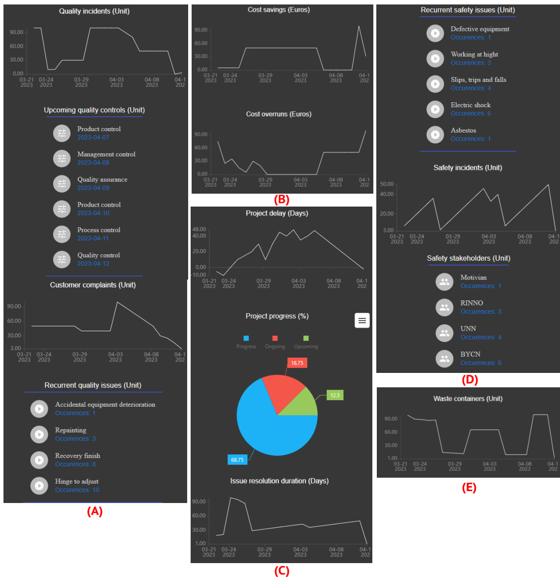
Figure 4: The RDT platform KPIs' dashboard for (A) Quality (B) Cost (C) Scheduling (D) Safety (E) Environment.
