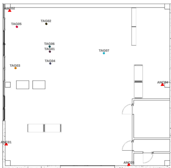
Figure 5 - Localization tag inside the DC3 lab during tests.
