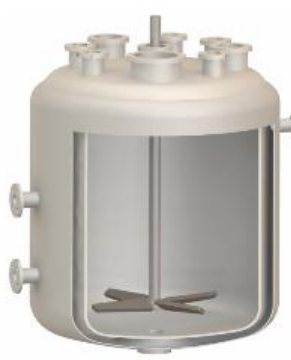
(b) Typical pharmaceutical reactor
