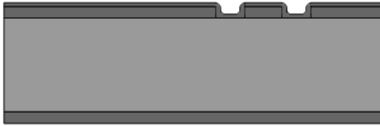
(b) 30 nm thermal SiO 2 layer for implantation
