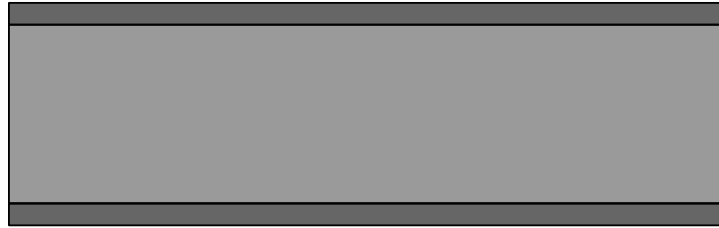
(b) Bottom wafer with 500 nm SiO 2 on both sides
