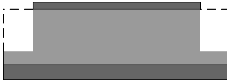
(d) PECVD of 2.5 \mu\text{m} on top side, 275 \mu\text{m} DRIE of inlet and outlet, and PECVD of 6 \mu\text{m} on bottom side on bottom wafer
