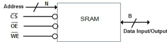
Figure 2.15: SRAM block diagram
