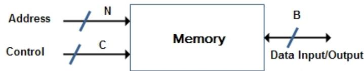
Figure 2.13: Memory block diagram
