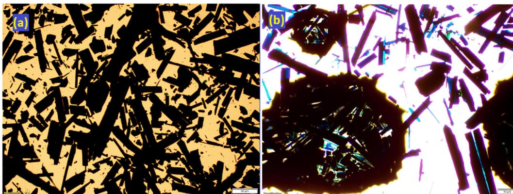
**Figure 4.** Optical microscopic images of (a) asphaltene in hexane and (b) asphaltene in hexane along with 0.01 mL of [BMIM][PF<sub>6</sub>] IL. The length scale of each optical image is 50  $\mu\text{m}$ .
