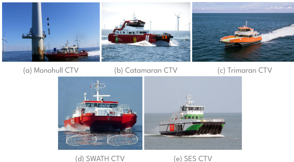
Figure 4.1: Different CTV types, (a) (J. Jiang, 2020), (b) (Dixon, 2021), (c) (Snyder, 2023), (d) (Bluebird Electric, n.d.), (e) (Cooke, 2015)
