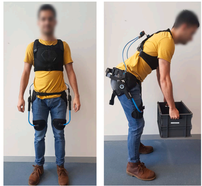
Fig. 1. Participant wearing the back-support Laevo Flex exoskeleton. The exoskeleton is a passive device which transfers loads from the lower back to the chest and thighs. The delivered assistance is provided by spring-like mechanisms acting around the trochanter major (hip joint). Spring mechanisms store energy in the bending down phase of the movement, which is (partially, as a result of hysteresis) returned to the user in the lifting phase. The smaller the torso-thigh angle, the higher the moment produced by the exoskeleton. The actuator strength was set to 70% (medium assistance) for all participants and lifting conditions.
