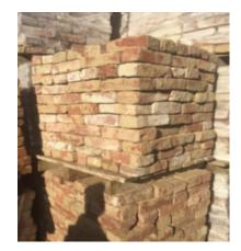
Figure 45 Used bricks to be reused. Some usage damage on the product can be appreciated. (Bouwfonds Property Development, 2019)
