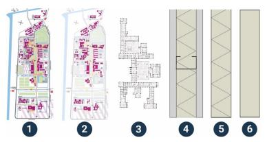
Figure 7 Example of the different levels to classify buildings. (1) Terrein: Campus TUDelft, including green area and infrastructure; (2) Complex: Faculties and facilitaire buildings; (3) Structure: Architecture Faculty; (4) Element: internal wall within structure; (5) Product: insulation board; (6) Material: Stone wool; seventh level not illustrated (Author)
