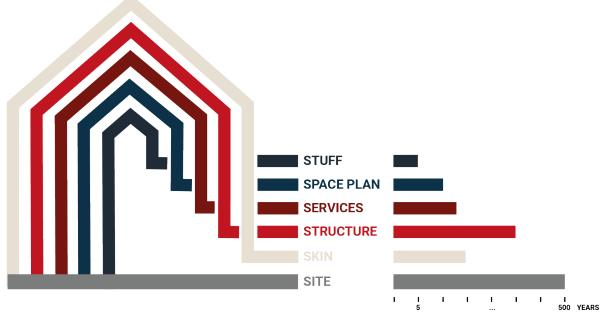
Figure 8 6s model according to Brand (1994), each layer has a different lifespan stuff (5), space plan (10), services (15), skin (20), structure (100) and site (500). Illustration adapted by author.
