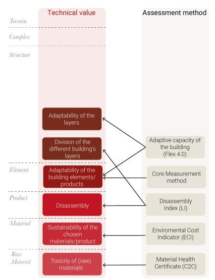
Figure 10 Relationship between the aspects of the technical values per building scale and possible assessment method. The assessment methods are independent from the building scale (Author)
