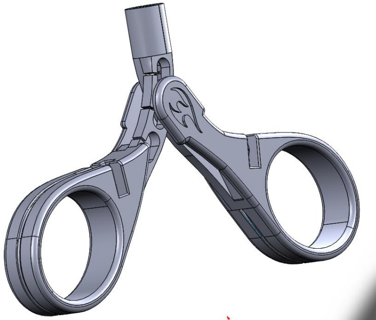
Figure G.1: Digital drawings of combined control handle halves.
