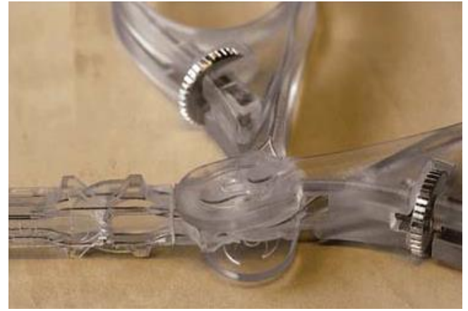
Figure 19: Control handle as used in the DragonFlex, existing out of multiple parts, connected via gear wheels. Adapted from [10].
