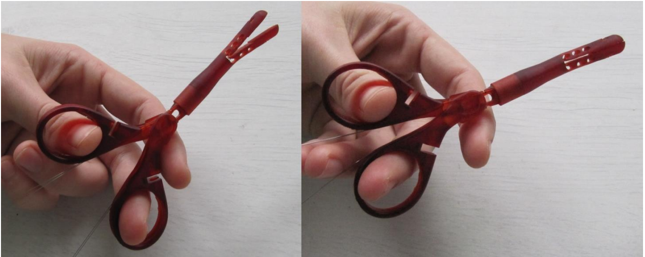
Figure 22: Separate grasping forceps part and control handle part attached and connected by a (non-fixated) control wire. Left: instrument opened, right: instrument closed.
