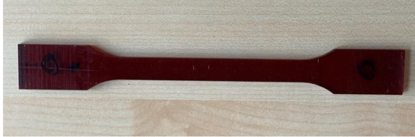
Figure A.1: Dog bone as used in five dogbone tests.
