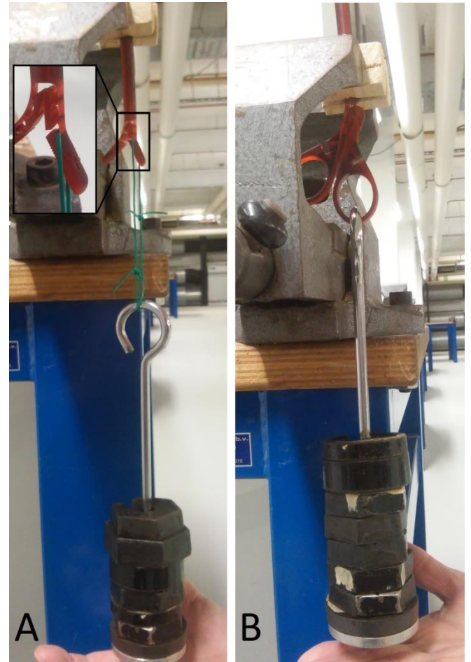
Figure 31: (a) Tensile test on the grasping forceps side of the MonoFlex, (b) tensile test on the control handle side of the instrument.
