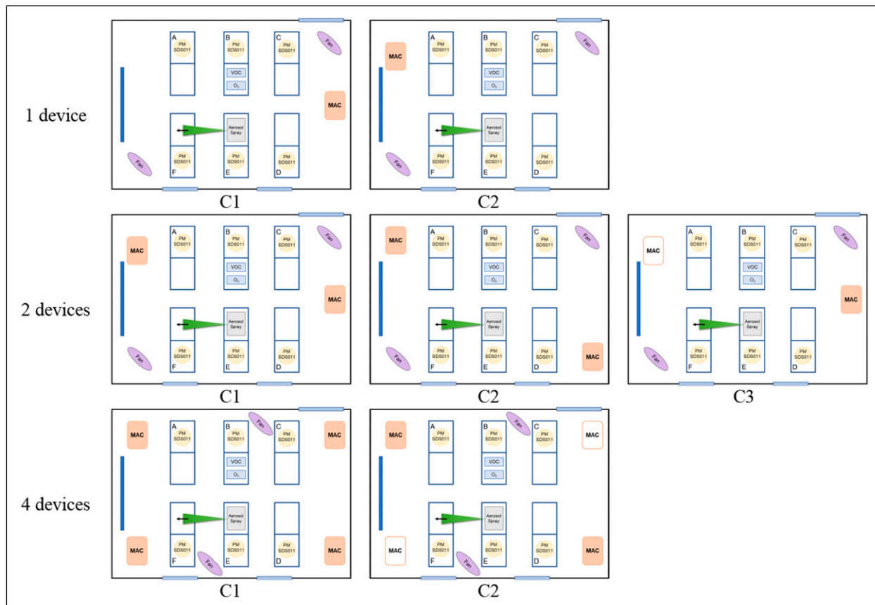
Figure 6. Configurations of the mobile air cleaners for the aerosol decay test: view from the top of the experience room, where A, B, C, D, E and F represent the tables, the dark blue rectangle represents the smartboard, and the light blue rectangles represent the door (top) and windows (bottom).
