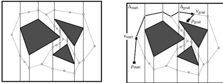
Figure 3.7: Road map of space with obstacles. Source: [De Berg et al. \(2008\)](#)
