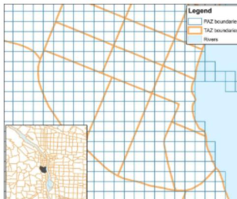
Figure 2.2: PAZs represented by a regular grid with a cell of 80x80 meters.
