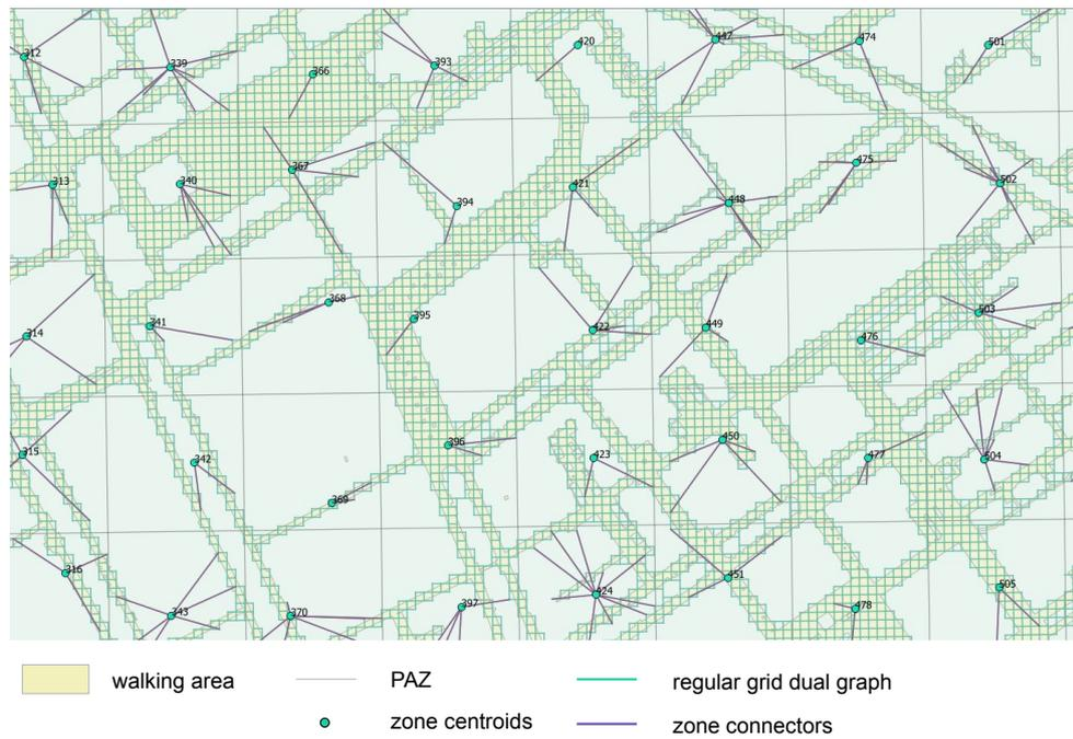
Figure 5.25: Zone connectors for regular grid dual graph created using DBSCAN to select graph points
