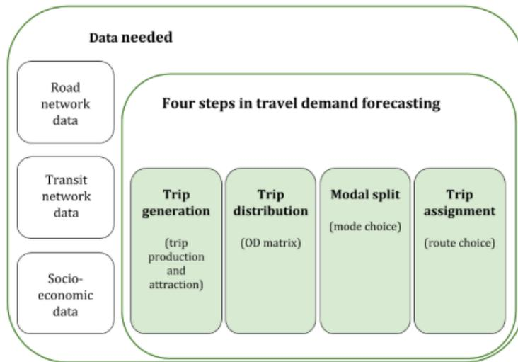
Figure 1.1: Components of the four step model (Woldeamanuel, 2016)
