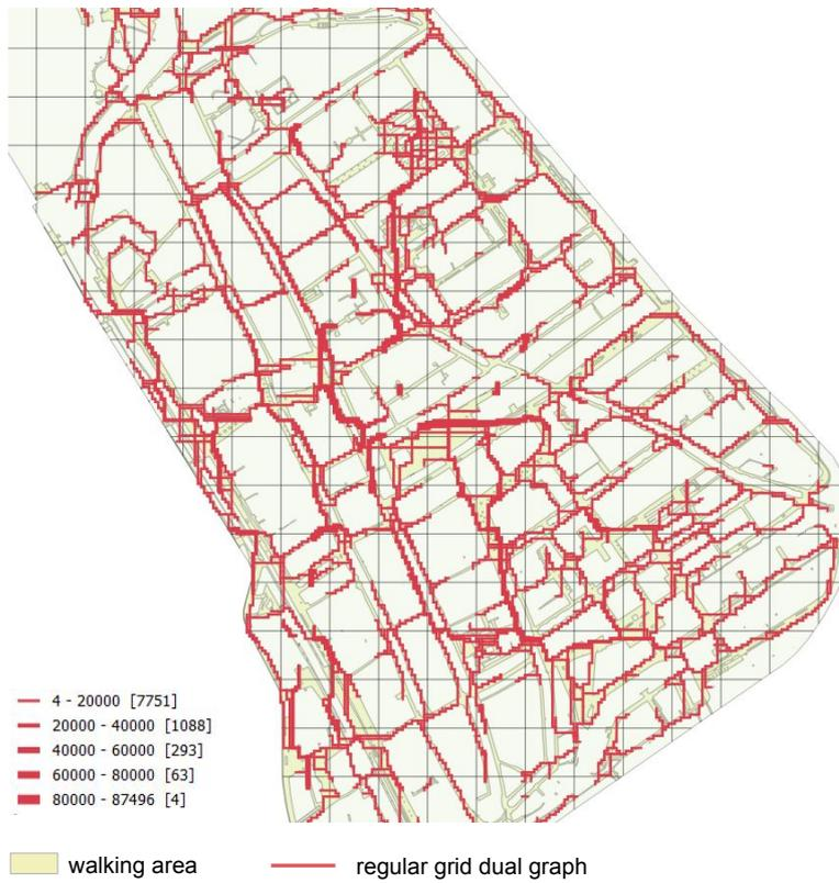
Figure 5.27: Assignment of trips on the network; regular grid dual graph
