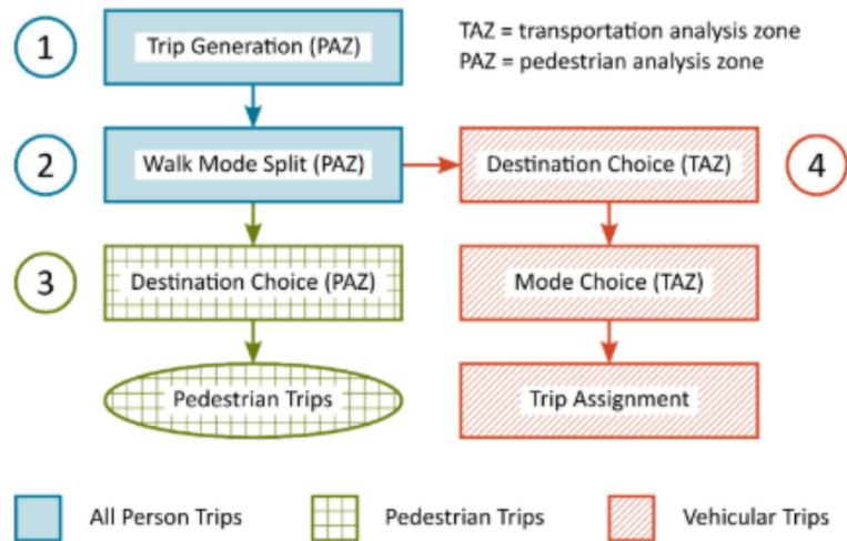
Figure 2.1: Conceptual diagram of proposed pedestrian modeling framework.
