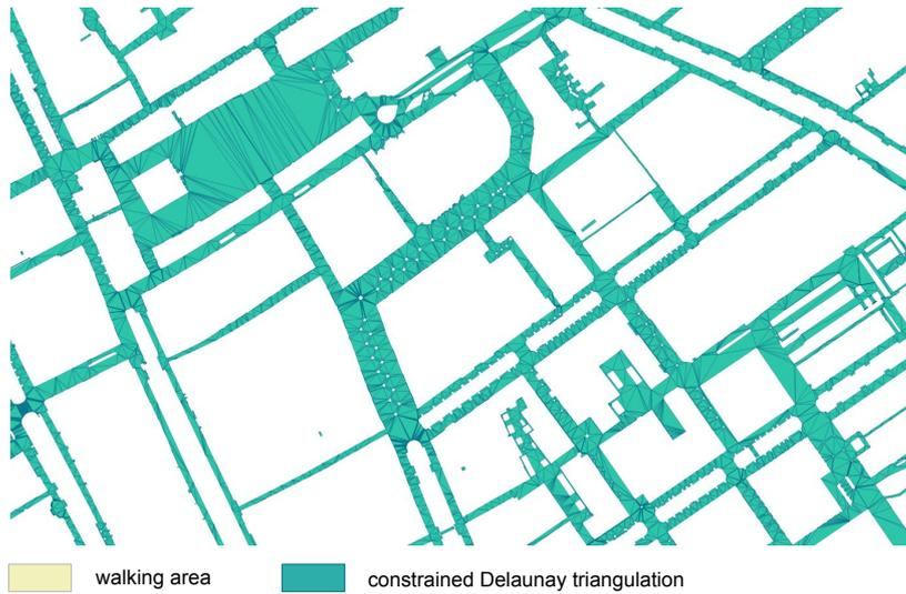
Figure 5.3: Walking space discretization with polygon triangulation
