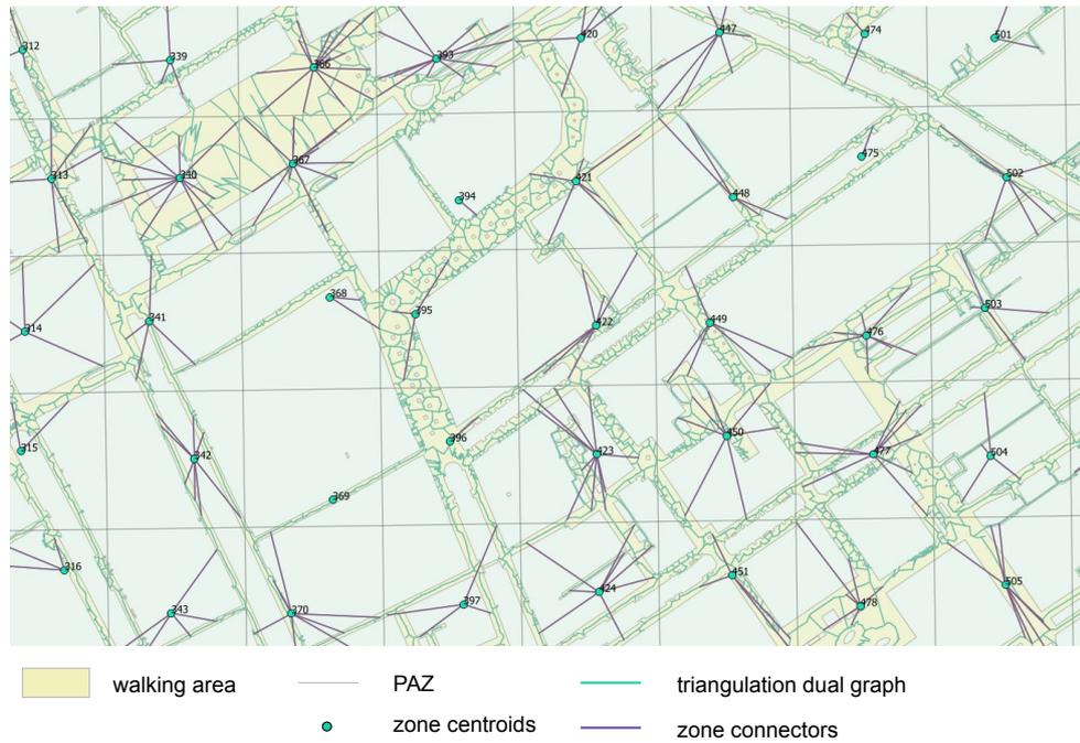
Figure 5.24: Zone connectors for triangulation dual graph created using DBSCAN to select graph points
