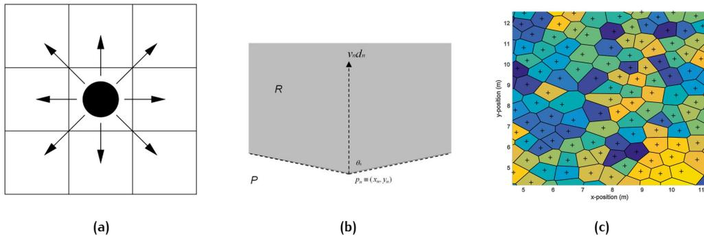
**Figure 3.1:** Space modeling techniques. (a) Cellular automata model. Space is discretized with cells. Source: [Schadschneider \(2001\)](#), (b) Space that corresponds to each individual based on direction and visual field. Source: [Antonini et al. \(2006\)](#). (c) Voronoi diagram of pedestrians. Each cell corresponds to a single pedestrian. Source: [Hoogendoorn et al. \(2017\)](#)
