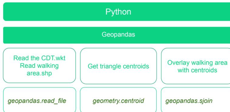
Figure B.2: Workflow of final triangulation inside walk area polygon
