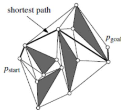
Figure 3.9: Visibility graph. Source: De Berg et al. (2008)
