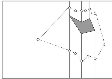
Figure 3.10: Trapezoidal map and road map on a polygon with one obstacle
