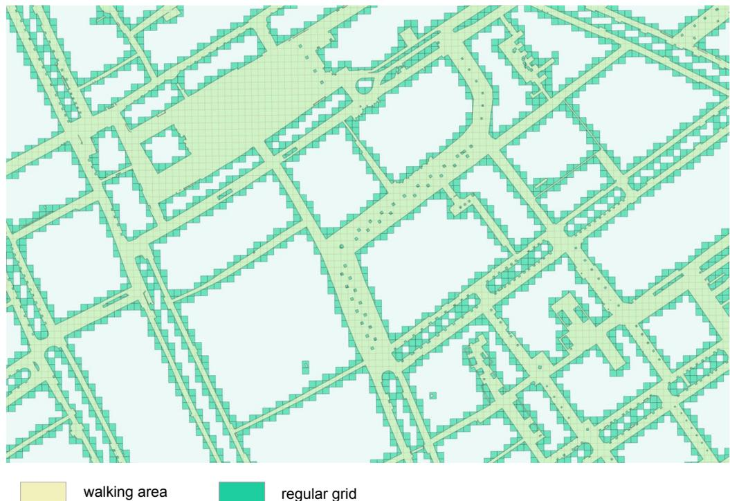
Figure 5.9: Space discretization with regular mesh of  $5 \times 5m$
