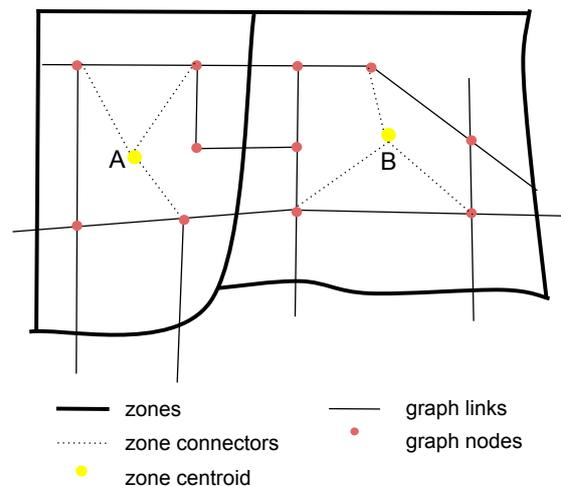
Figure 2.4: Use of zone centroids and zone connectors to inject the trips of the OD matrix to the road network in the example area
