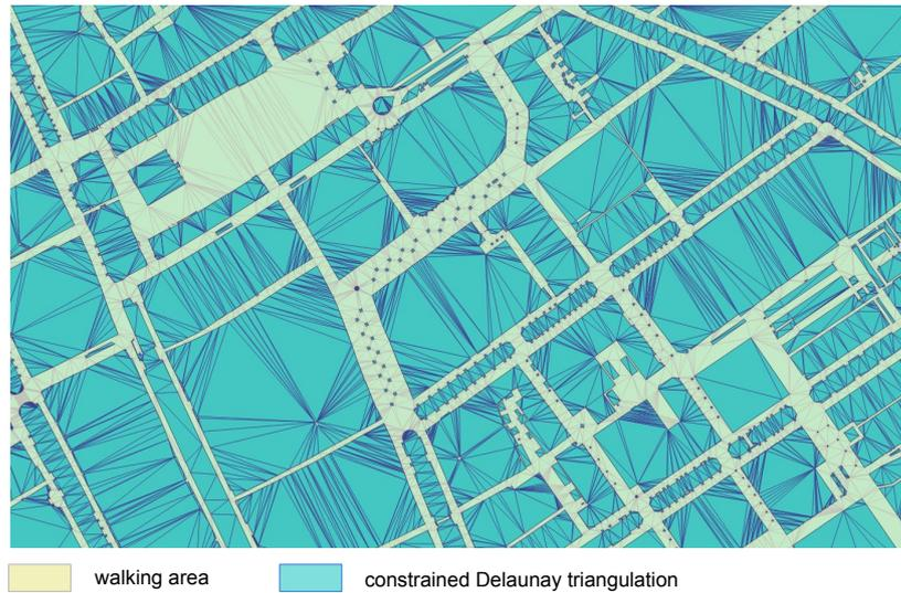
Figure 5.2: Constrained Delaunay triangulation in application area
