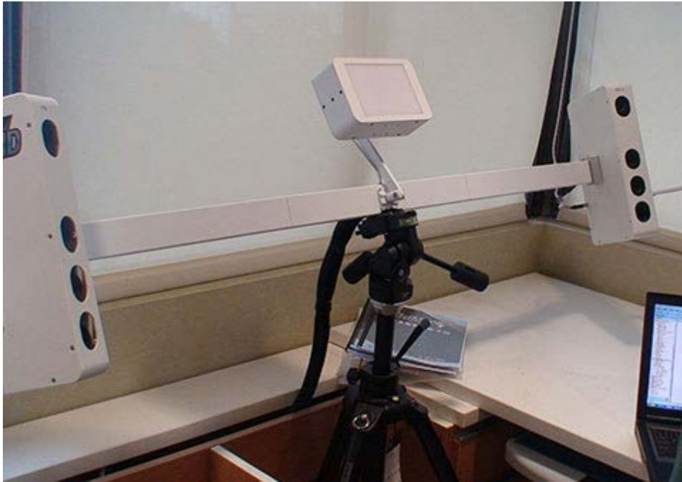
Fig. 3f: 3dMDface scanner with 2 camera modules and the LED system visible.
