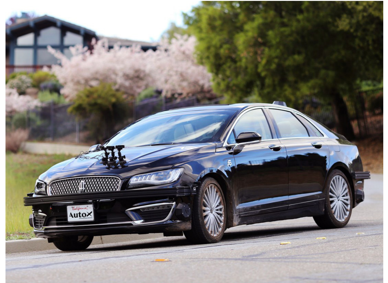
'AutoX Has Built a Self-Driving Car That Navigates with a Bunch of $50 Webcams'
