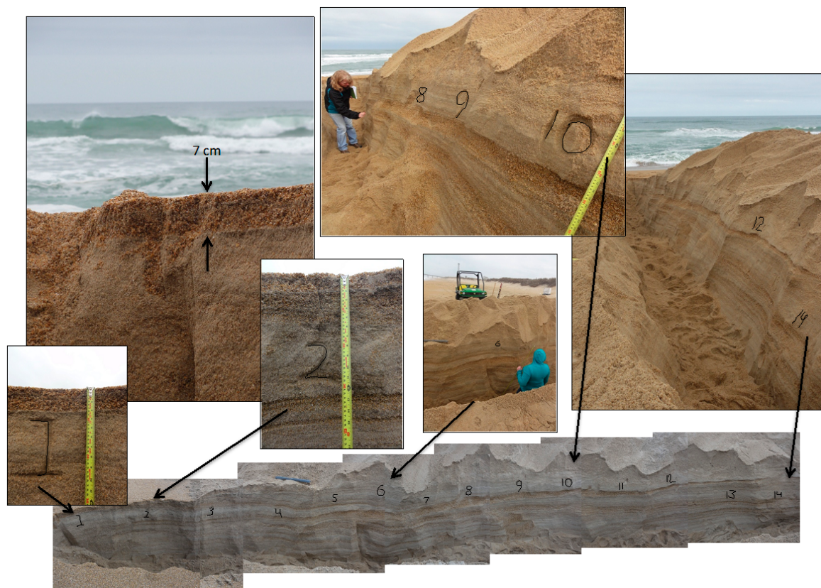
Figure 6. Images of the cross-shore trench that was dug near the end of the experiment. The bottom image is a compilation of multiple images, showing the whole trench. The other images show details (like layer thickness and extent) at various locations in the trench. Note the numbers scratched in the sand wall (and outlined in black) of the trench approximately every meter for reference.
