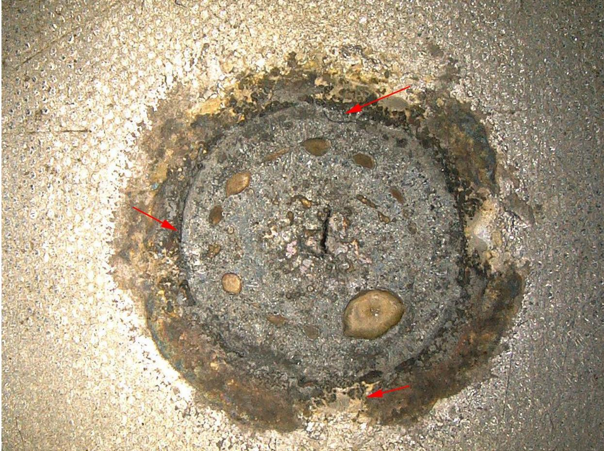
**Figure 4.21:** Optical micrograph of an LBW dog-bone sample, loaded to 80% of yield strength, loading direction left to right, welded using 800W beam power defocused to 1 mm for 2 s, with circumferential features marked.
