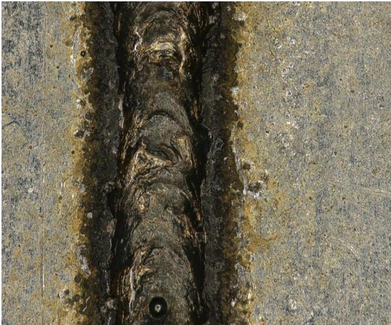
**Figure C.2:** Keyence digital micrograph of linear weld welded at 1 kW at a speed of 10mm/s under 100% ys tensile load.
