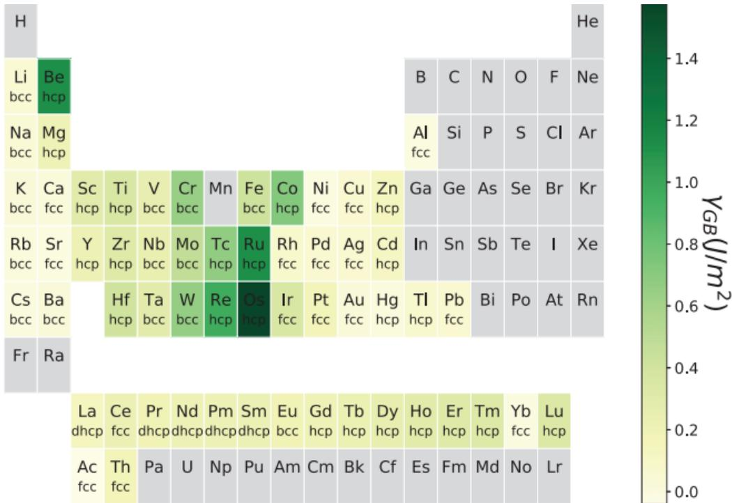
**Figure 5.2:** Average grain boundary energies of elemental metals, including their crystal structure, as determined through DFT calculations [47]
