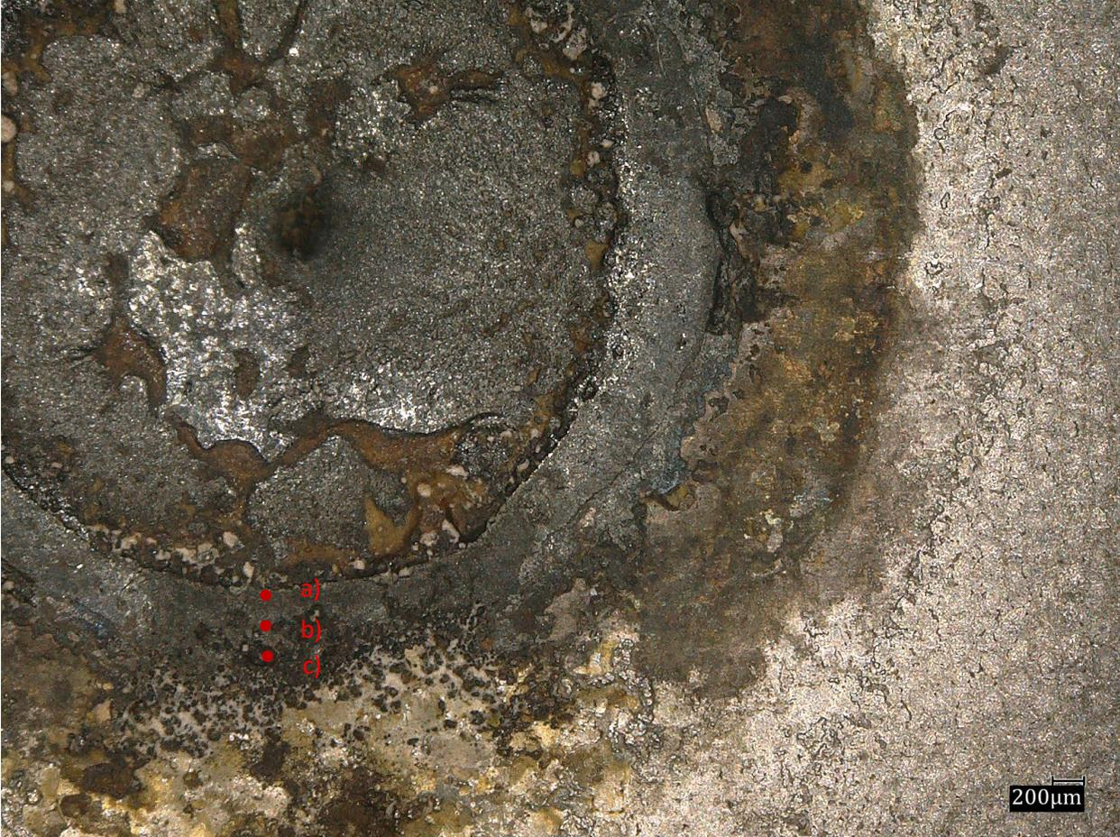
**Figure 5.4:** LBW Spot weld surface, welded at 800 W laser power for 2 s with a spot diameter of 1 mm. The approximate probed locations for FEA are marked. a) First location, called inner edge HAZ, b) second location, called middle of HAZ, c) third location, called outer edge HAZ
