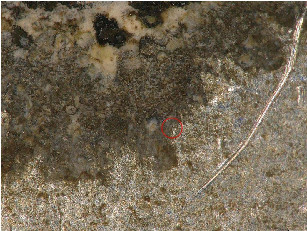
**Figure C.4:** Keyence digital micrograph of top surface of laser welded sample welded at 200 W, beam defocussed to 7mm for 10 s at 100%  $\sigma_s$  tensile load, showing a possible crack feature.
