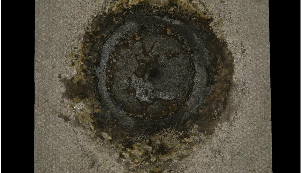
**Figure C.1:** Keyence digital micrograph of the surface of a LBW sample welded at 800W, with the beam defocused to 1mm for 2s under 100% ys tensile load.
