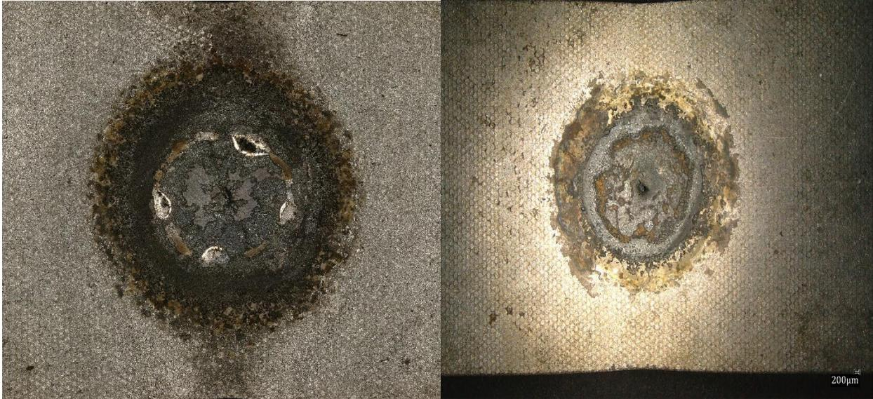
**Figure C.3:** Keyence digital micrograph of the bottom surface of laser welded samples. Left image: welded at 800 W, beam defocussed to 1mm for 2s at 100%  $\sigma_s$  tensile load. Right image: welded at 800 W, beam defocussed to 1mm for 2s at 800%  $\sigma_s$  tensile load.
