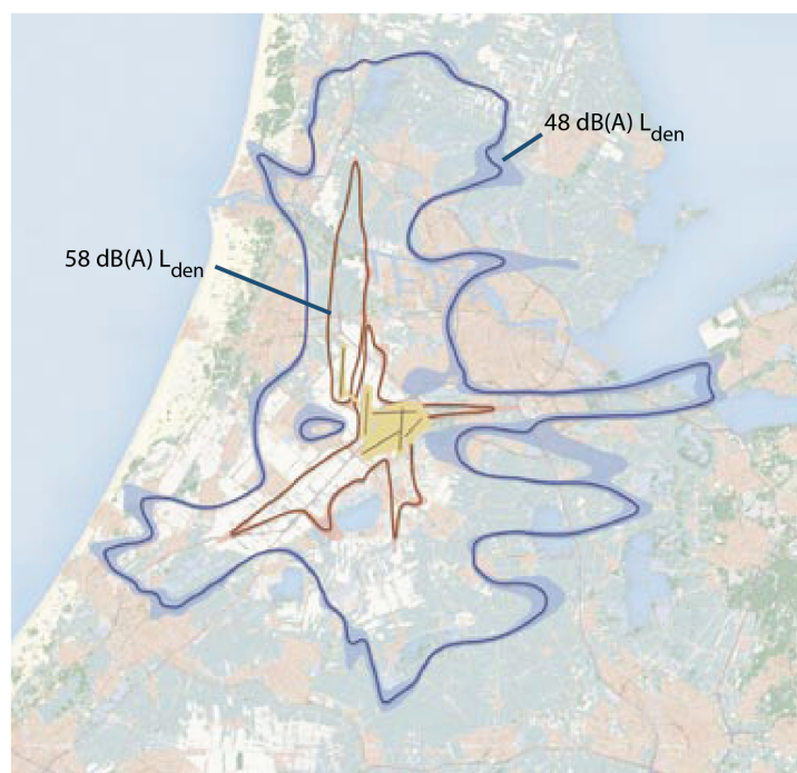
Figure 3.6: Noise contours of equal L_{den} constructed with a theoretical model of AAS. Retrieved from [2]
