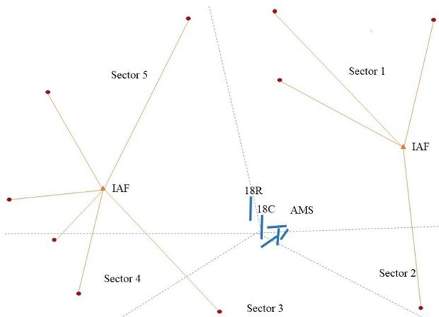
Figure 5: The fixed arrival route and the sectors of the Dutch airspace.
