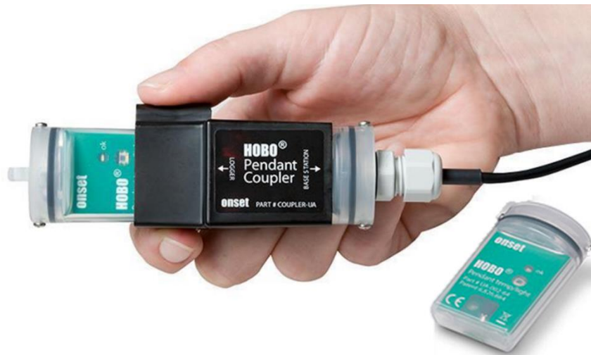
Figure 30 – Data logger for temperature and light used in the Erasmus MC with the base station to read the recorded data [24, 25].
