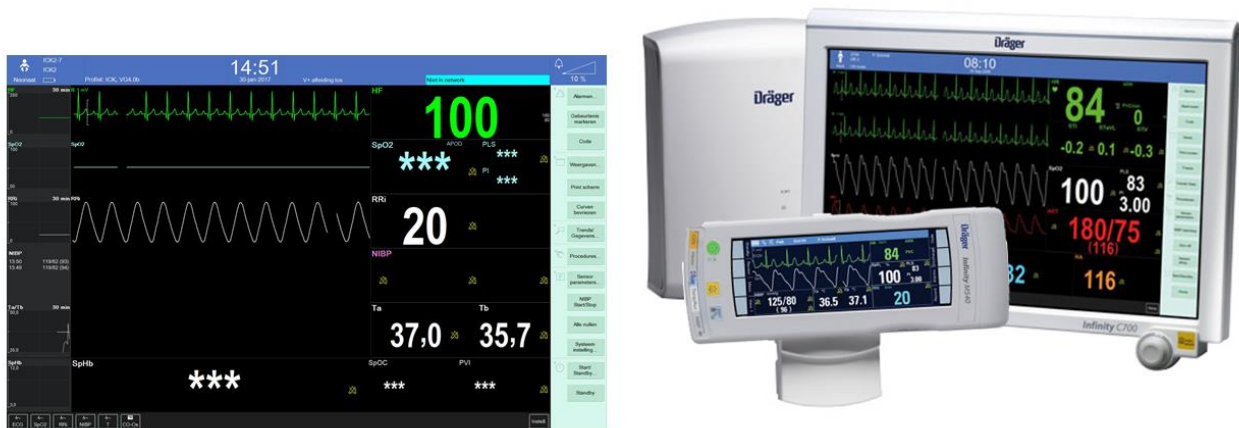
Figure 26 – Patient monitor and display monitor used in Erasmus MC (right, [22]) and an example of the screen display in simulation mode showing the central and peripheral temperatures (right).
