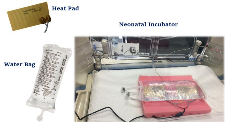
Figure 33 – Initial experimental setup showing the water bag and heat pads and how they were positioned inside the neonatal incubator.
