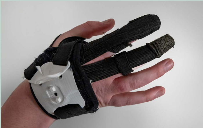
Figure 52: promosing prototype, the elastic bands are modular and good counterforce.
