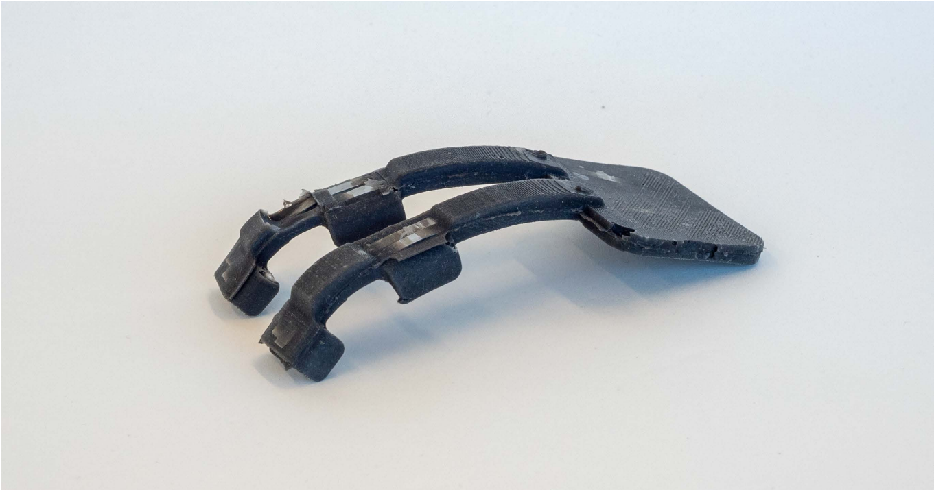
Figure 83: Splints with springsteel 0,2 mm thick and 4 mm wide. Tested if less spring steel will also provide enough damping, this was not the case. see appendix 32, for the making proces.
