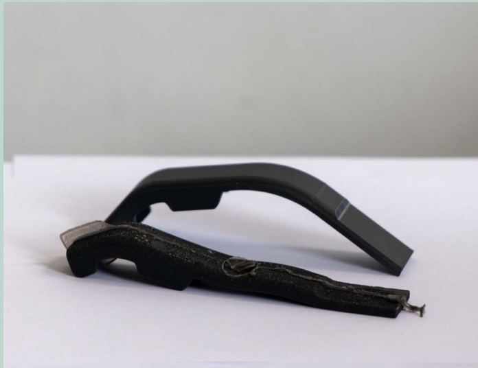
Figure 46: splint in front from silicone and in the back from 3d printing
