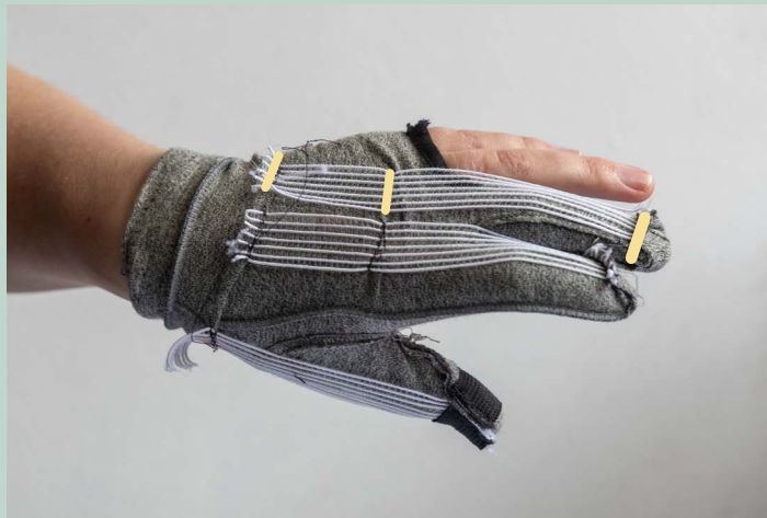
Figure 51: third prototype elastic bands. Did not give a lot of counter force. The limit stretch from the glove fabric, limited the elasticity.
