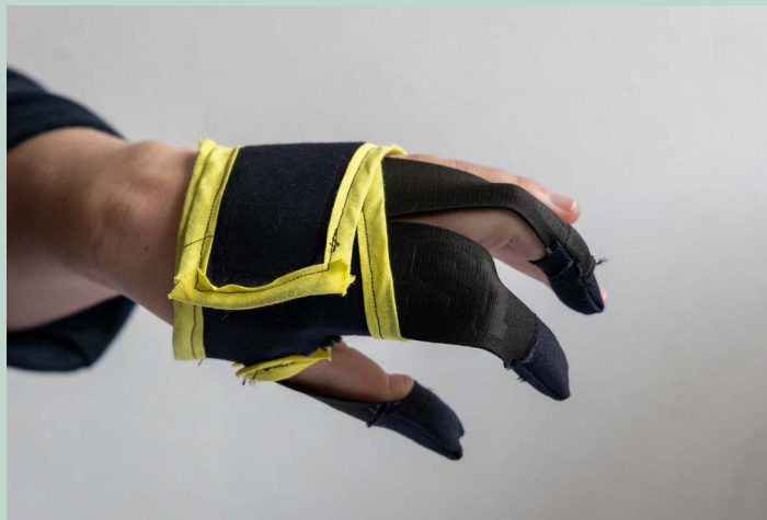
Figure 50: second prototype elastic bands. Elastic too stiff and fabric around hand not stabile
