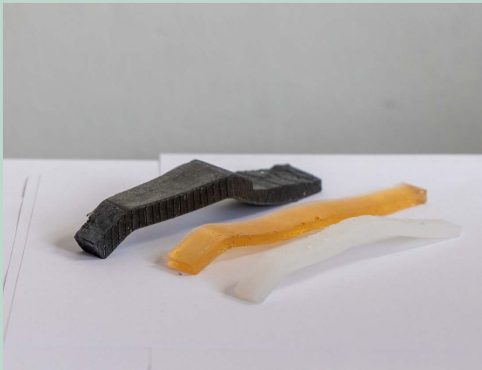
Figure 44: silicone splints, dark splint (shore 40), yellow/orange splint (shore 60, white splint (shore 25)
