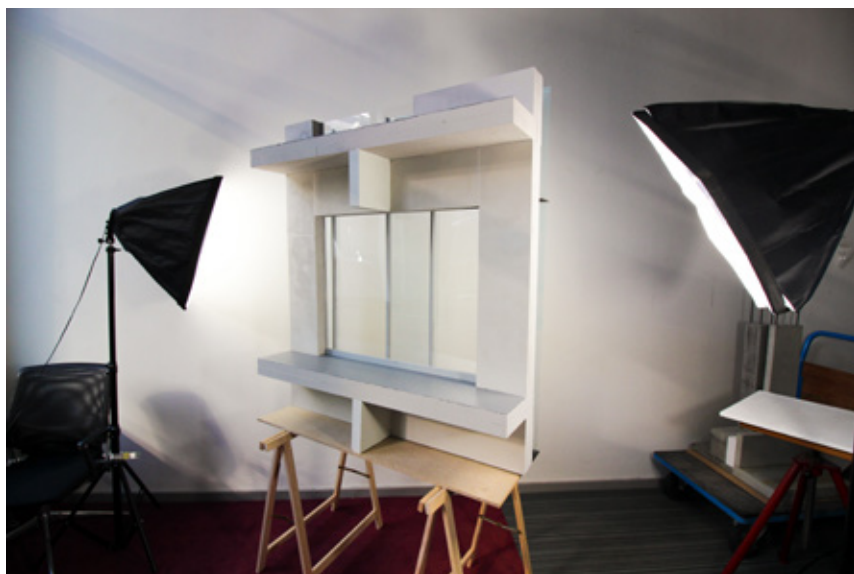
Fig. 11.10 Foam and polyester model of a fragment of the facade by Robbrecht and Daem, scale 1:5, by Mees Wijnants and Tommaso Tellarini. Photograph: Mees Wijnants and Tommaso Tellarini.
