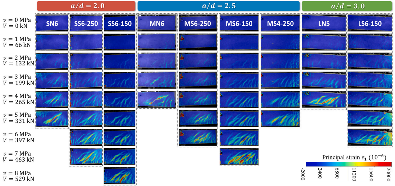
Fig. 19. Shear crack propagation in selected beams (left shear span) captured by 3D-DIC system.
