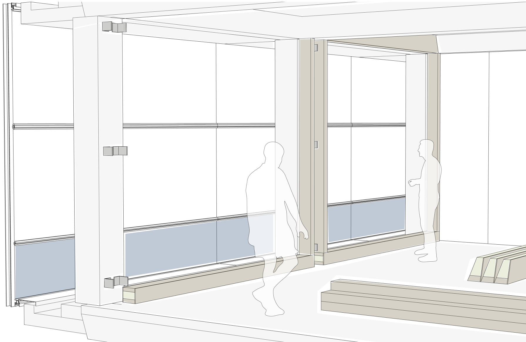
Step 2.1 | Place surrounding frame to existing construction
