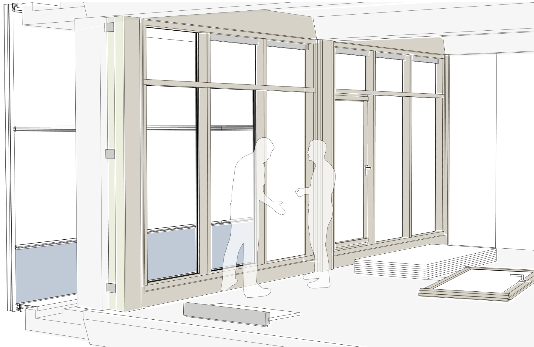
Step 2.4 | Install curtain wall glass and door elements
