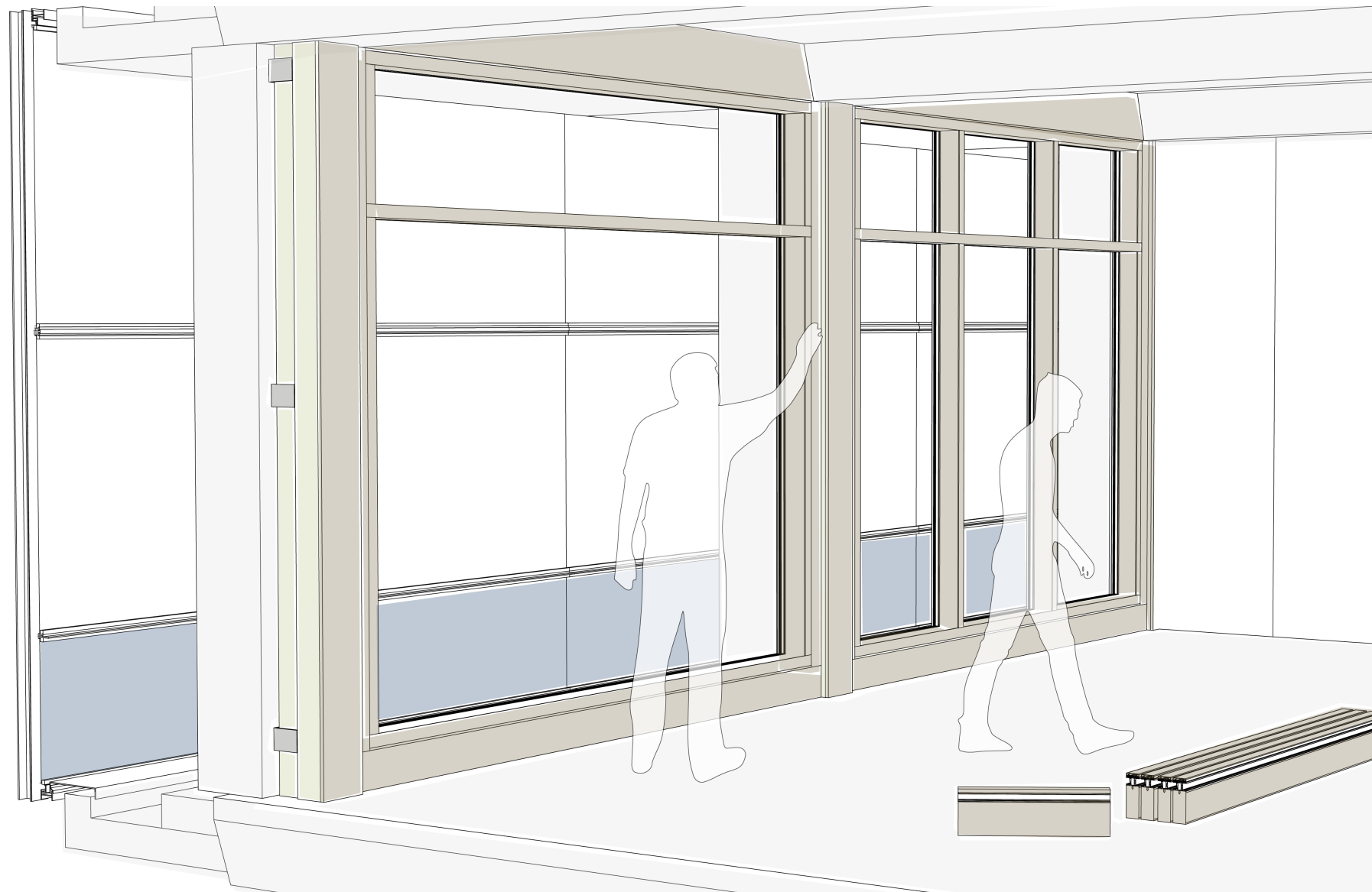
Step 2.3 | Place curtain wall frame divisions
