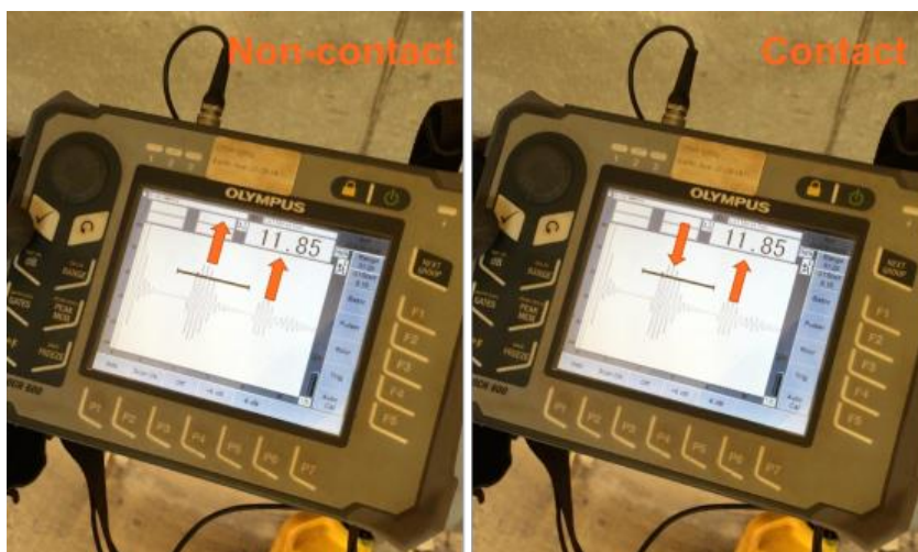
FIGURE 5. DIFFERENCE NON-CONTACT SITUATION (LEFT) VERSUS CONTACT SITUATION (RIGHT)
