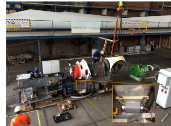
(c) Close up accelerometer
