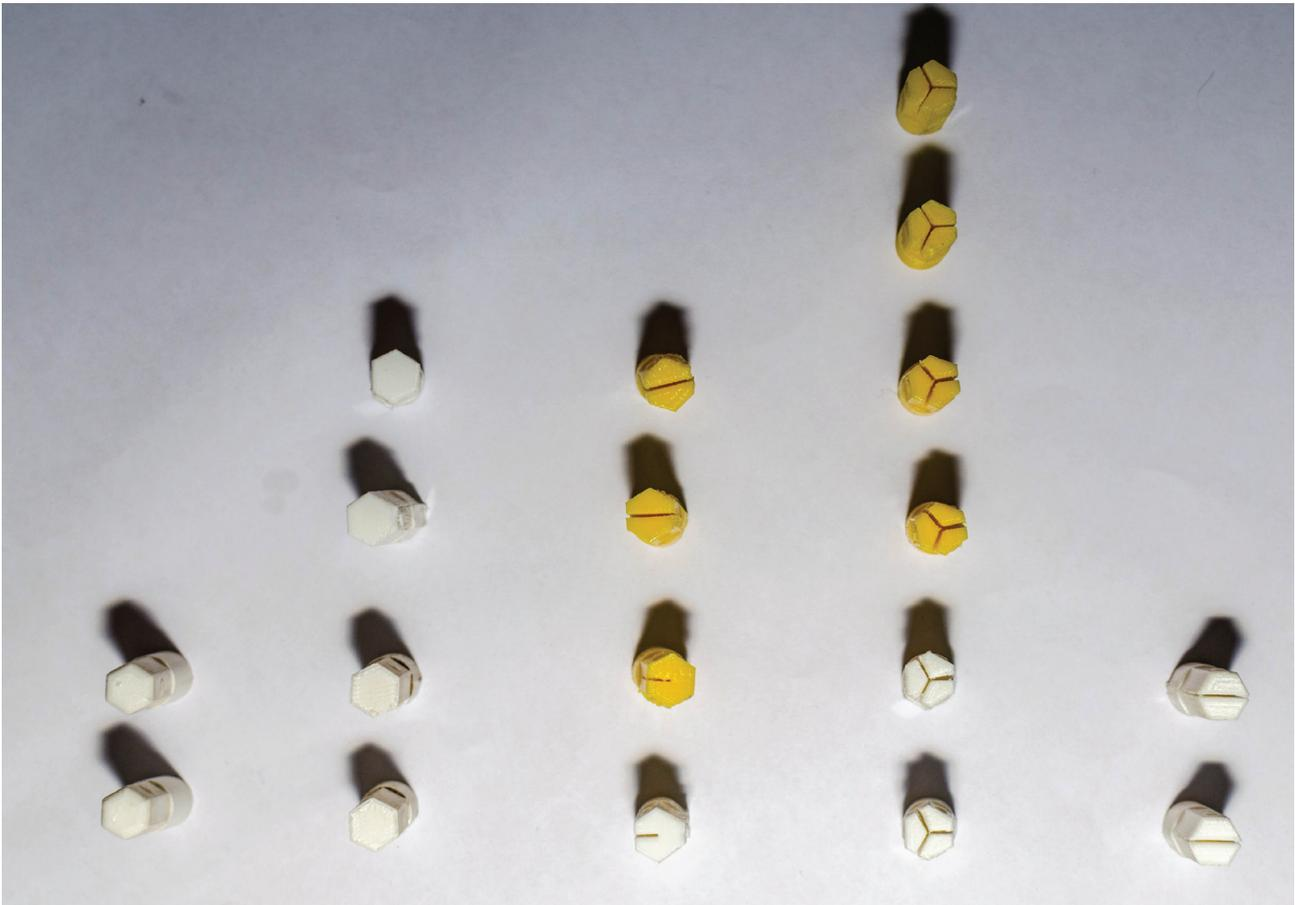
Figure 32: Multiple iterations of axes to create one that is attachable, keeps attached to and is removable from the wheel. Oldest to newest iterations from left to right.
