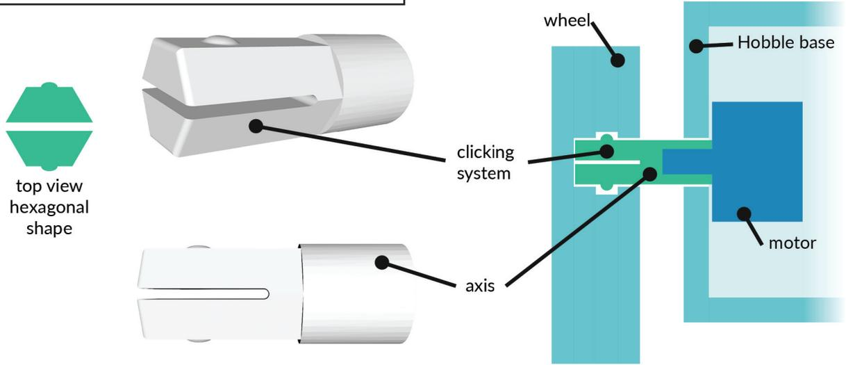
Figure 31: Clicking system with two rounded extrusions that fit in gap inside the wheel.
