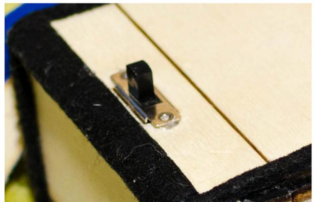
Figure 40: Prototype on/off switch. Not clear on what side is on or off.
