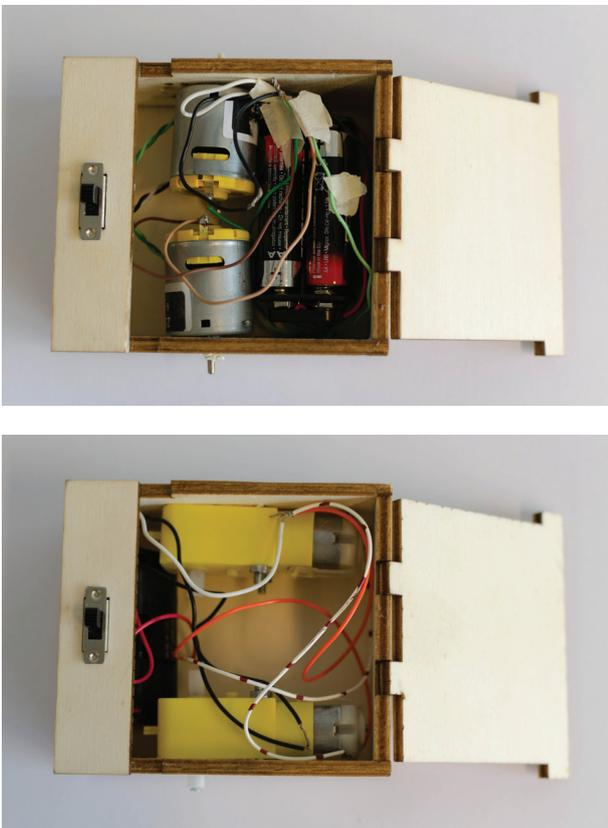
Figure 24: Old motors (above) replaced with newer higher torque and lower speed motors (below).
