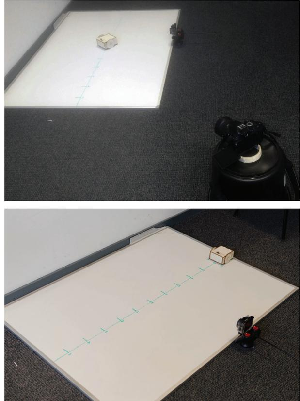
Figure 29: Two angles of the test setup for the wheel tests. Flat surface guide track, two cameras (side and 3/4 view).
