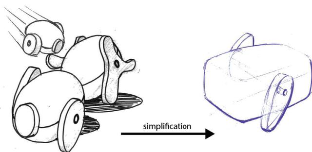
Figure 18: Simplification of the walking idea into a buildable prototype.
