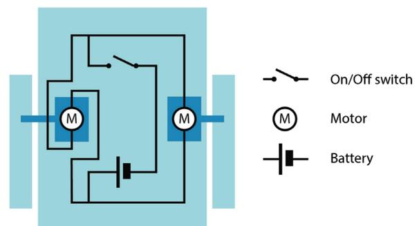
Figure 19: Electrical scheme connecting the battery, the switch and the two motors parallel.
