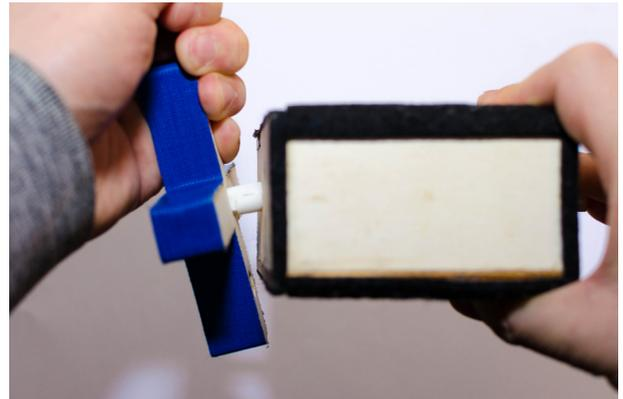
Figure 39: Pull and remove wheel diagonally from the axis
