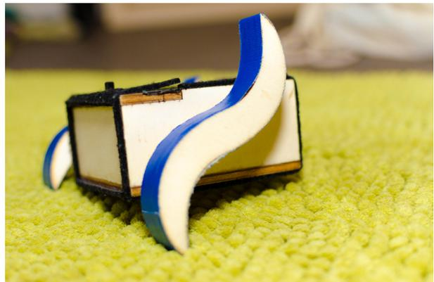
*Figure 41: Deep-pile carpets were troublesome for Hobble, especially for the backside of the base.*
