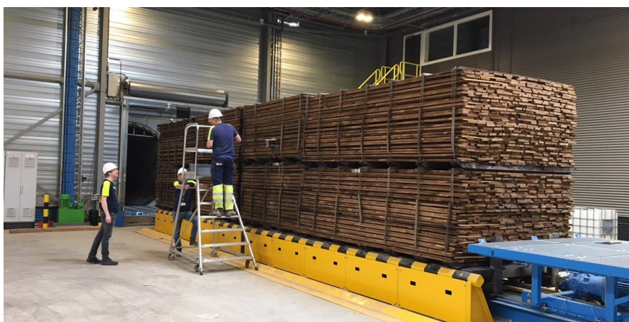
Figure 3.14: Acetylated batch of Radiata pine (Accoya, 2024).
