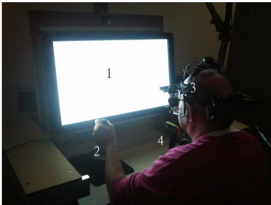
Figure 5-1: A subject in the measurement setup at the EMC consisting of a screen (1), a modified HOTAS Warthog joystick (2), an infrared eye tracking system (3), and a chin rest (4).
