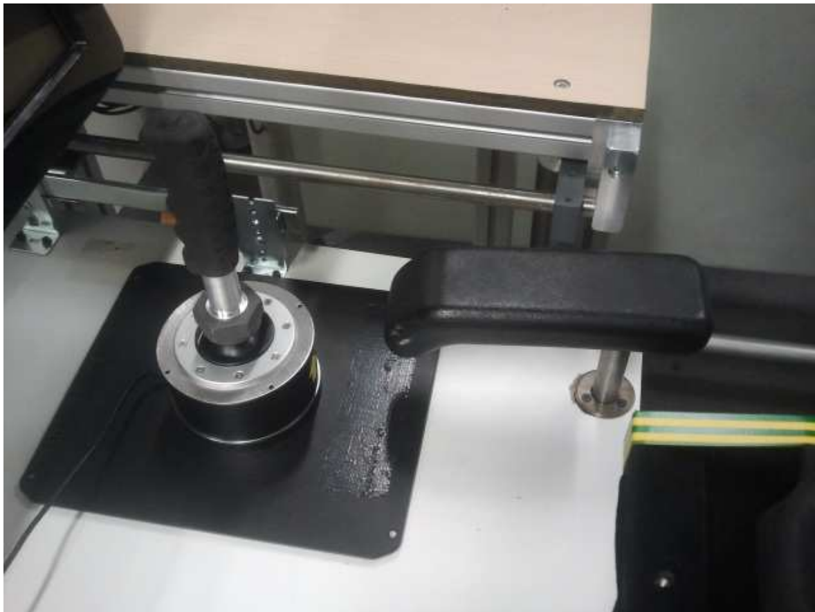
Figure A-1: Modified HOTAS Warthog joystick in the EMC setup.
