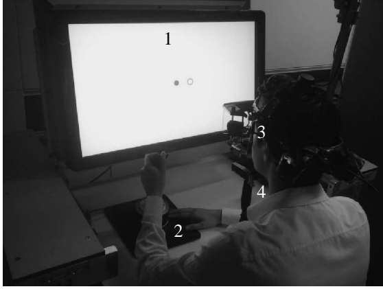
Figure 1: A subject seated in the measurement setup consisting of a screen (1), a modified HOTAS Warthog joystick (2), an infrared eye tracking system (3), and a chin rest (4).
