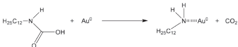
Figure 2.3: Dodecylcarbamic acid decomposition into dodecylamine and carbon dioxide. Dodecylamine interacts with gold nanoparticle surfaces and stabilizes them.
