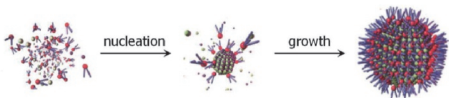
Figure i.1: Schematic of the nucleation of metal nanoparticles (green), and their stabilization by capping ligands (red and purple).
