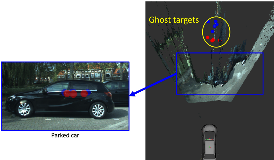
Figure 2.13: Real world examples of ghost targets. On the left, targets are projected into the camera view. On the right is a top view of the scene with the stereo camera point cloud. Notice that the targets are farther away from the ego-vehicle (bottom of top view) than the parked car. This is because the radar signal is reflected off the large flat slide of the parked car, and the radar sensor is detecting the ego-vehicle itself. The colors of the targets indicate the outcome of the classification algorithm presented in Chapter 5. Namely, blue targets have the car class assigned to them, red targets have the cyclist class assigned to them.
